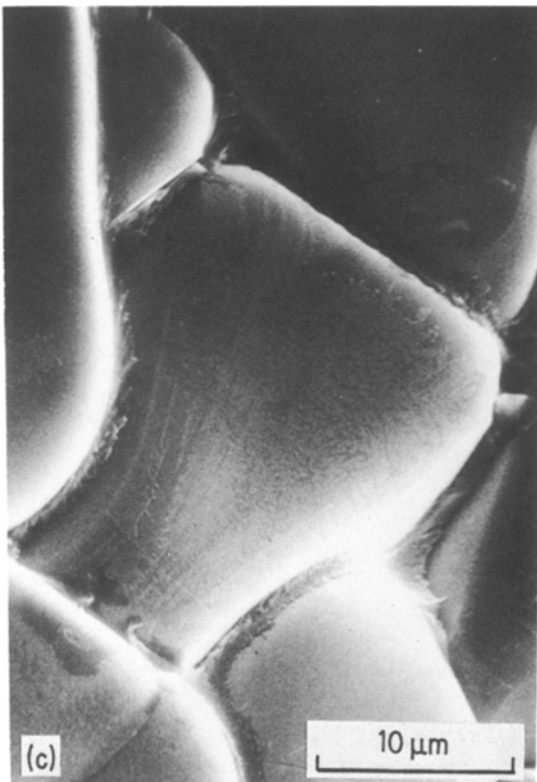
Figure 5 Different second phase morphologies in 0.5 mol % Sr composition: (a) large, transparent particles, 1400° C 2 h and annealed at 1200° C 24 h (b) discrete, GB particles, 1400° C 2 h quenched to room temperature followed by 1200° C 2 h and (c) continuous GB second phase, 1400° C 2 h and annealed at 1250° C 20 h; all SEM micrographs.
