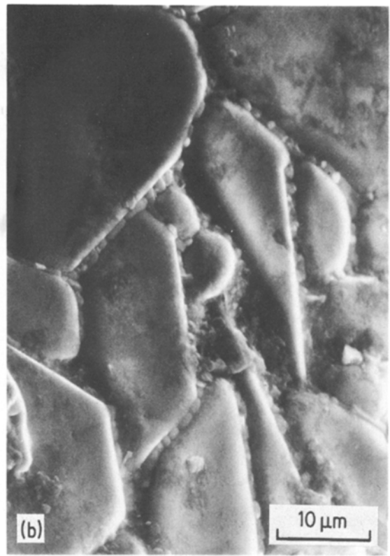
Figure 5 Different second phase morphologies in 0.5 mol % Sr composition: (a) large, transparent particles, 1400° C 2 h and annealed at 1200° C 24 h (b) discrete, GB particles, 1400° C 2 h quenched to room temperature followed by 1200° C 2 h and (c) continuous GB second phase, 1400° C 2 h and annealed at 1250° C 20 h; all SEM micrographs.
